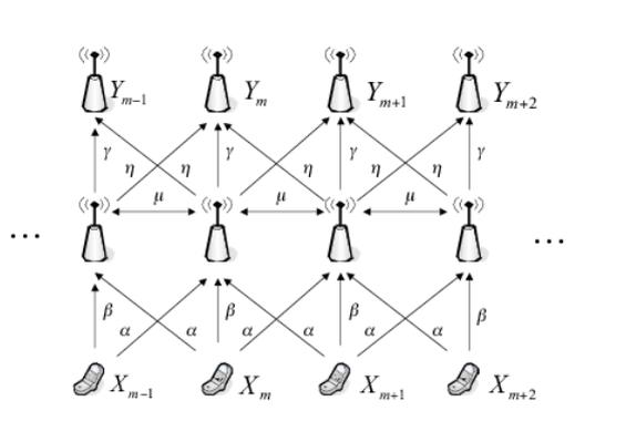
Grid-based models often cannot handle multicell networks analytically so Wyners Model can be used to simplify the methods in which researchers model and analyze these networks (Figure 6). Analytical and simplistic models such as these are in limited within Cellular communication networks. Some of Wyners
